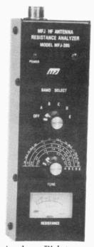
The MFJ-205 Antenna Resistance Analyzer™ lets you determine the feedpoint resistance of your antenna at its resonant frequency. It provides the same information as a conventional RF resistance bridge but is simpler and more convenient to use. The MFJ-205 also determines your antenna's resonant frequency and has a built in frequency generator with a frequency out jack.
